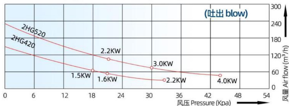
Compressor Selection Diagram 50HZ--压力选型图表50HZ
